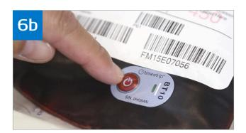
Firmly adhere the BT10 centered on the bottom third portion of the blood bag to get the most blood mass when sitting upright. Press the outer edges a few times to ensure proper adherence.
