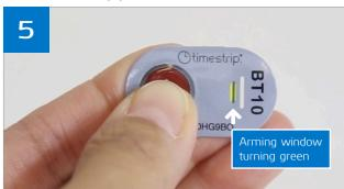
Firmly squeeze the activation button between thumb and forefinger until you feel a slight pop. The arming window should turn immediately from yellow to green.
