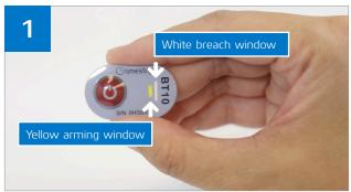
Select a Blood Temp 10 (BT10) indicator and implement a QC visual test to make sure it is not yet activated: the arming window should be yellow and the breach window should be white, signaling that the device has not yet been activated.
